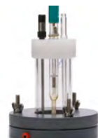
Flat Corrosion cell
