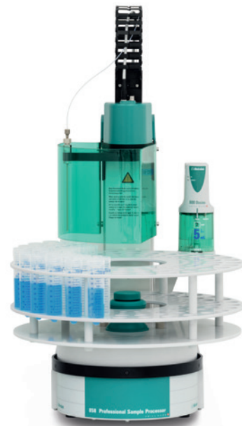
858 Sample Processor with Dosino for Sample Transfer
