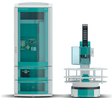
Figure 2. 940 Professional IC Vario with 947 Professional UV/VIS Detector Vario, 943 Professional Reactor Vario and the 858 Professional Sample Processor.
