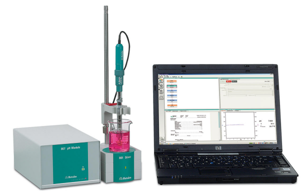
Figure 1. 867 pH Module controlled by tiamo software for performing standard addition.
