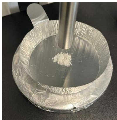
Figure 3. Precipitate recovered from the reaction and mounted on a BAC151B probe holder for Raman analysis.
