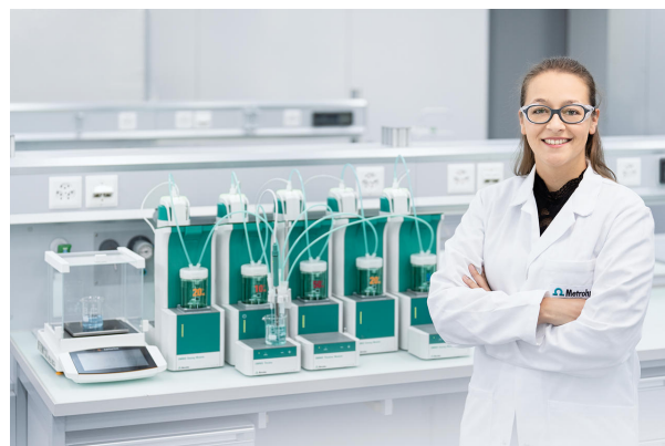
Figure 1. The OMNIS Professional Titrator with OMNIS Dosing Modules (shown here) are ideal for two-phase titrations of ionic surfactants when equipped with the Optrode M2.
