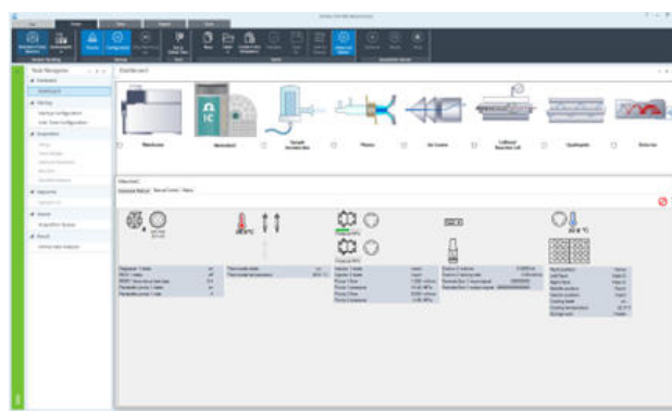
Figure 2. With the help of the Metrohm IC Driver 1.0, ICP-MS MassHunter (6.6090.100), full control of both devices (IC and ICP-MS) is possible in ICP-MS MassHunter as a single-software solution.
