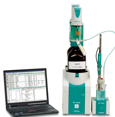
Figure 1. 905 Titrand with thiamine. Configuration of example for the determination of the titer of hydrochloric acid.
