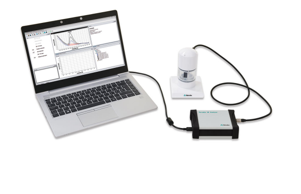
Figure 1. 946 Portable VA Analyzer (scTRACE Gold version)
