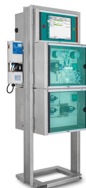
Figure 2. The Metrohm Process Analytics 2060 TI Ex Proof Process Analyzer.
