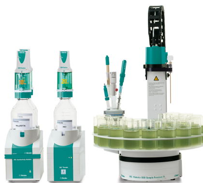
Figure 1. 815 Robotic USB Sample Processor XL with external titration vessel, 905 Titrand, and 856 Conductivity Module equipped with iAquatrode plus, combined Ca-ISE and 5-ring conductivity measuring cell for the analysis of tap water.
