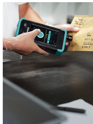
Figure 1. Finding contraband—from fentanyl to anthrax—in the mail is a very real issue. The ability of Raman to scan through paper is an invaluable asset.
