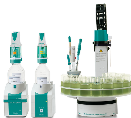
Figure 1. Example setup of a 815 Robotic USB Sample Processor XL with one external titration vessel, a 905 Titrando and 856 Conductivity Module equipped with iAquatrode plus, combined Ca-ISE, iAg-Titrode, and 5-ring conductivity measuring cell for the analysis of tap water.
