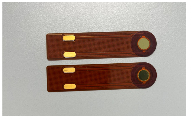
Figure 1. The crystal Pre (bottom) and Post (top) deposition.
