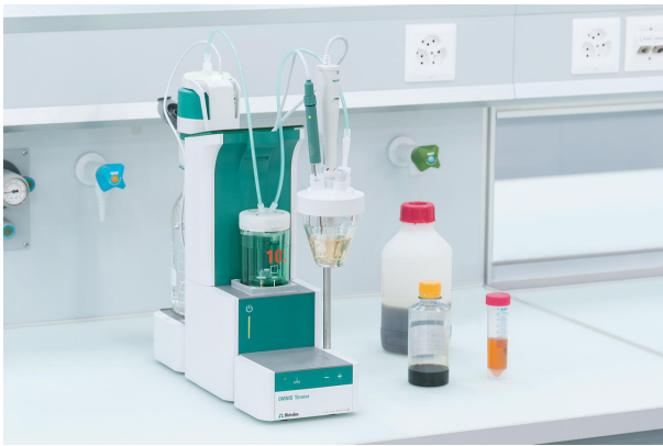
Figure 1. OMNIS Titrator setup for the thermometric titration. Data evaluation is performed with the OMNIS software.
