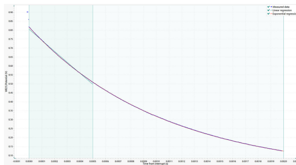
Figure 2. Measurement of ohmic resistance with current interrupt using a PGSTAT302N with the ADC10M.
