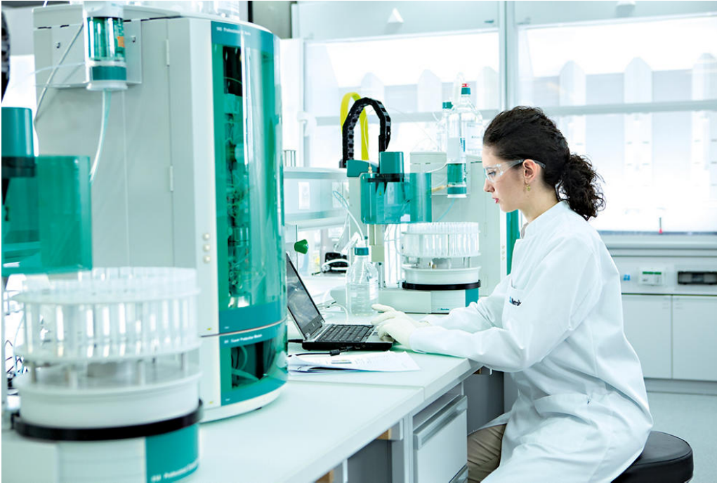
Figure 2. Ion chromatographs for laboratories (left) and for process analytics (right).
