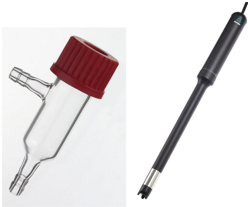
Hình 1. Used flow-through cell (left) and O 2 -Lumitrode (right).
