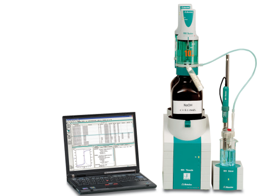
Figure 1. 905 Titrande with tiamo. Example setup for the determination of the iron content in iron ore.
