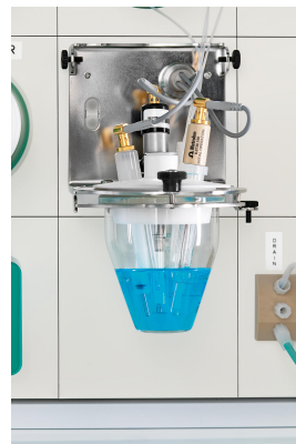
Figure 3. Close-up of the electrochemical cell in the 2060 CVS Process Analyzer.
